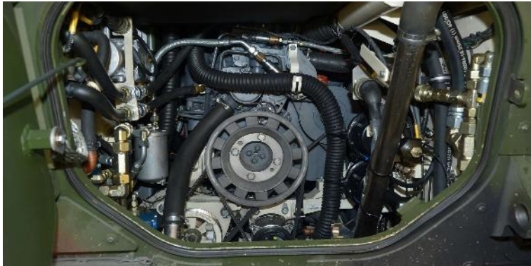
Diesel Engine for light military vehicles
